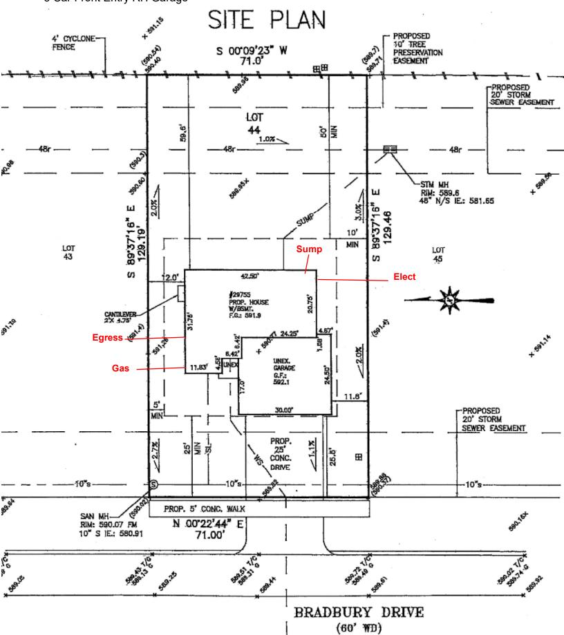
Site plan easement locations, house placement, surface concrete, grade elevations and dimensions are approximate and may vary during construction.
